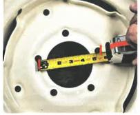
A bolt hole diameter measured with a
