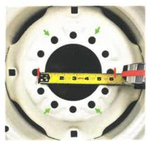
This wheel is an example of a 6 hole wheel that has 12 bolt holes. The 6 holes that are used to bolt the wheel to the hub are generally slightly larger and have a countersink. Measuring the bolt circle would be the same as the 8 hole wheel above. This wheel is a 6 Hole,6 inch Bolt Circle wheel.
